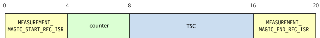
Figure 7.7: Data layout of the time stamp inserted in the MOST data
